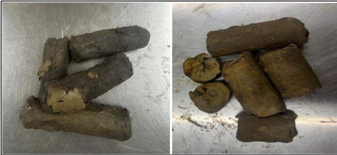
Figure 3: Stratum II Materials Left: S3B1 / S-2 (CL Materials) Right: S3B2 / S-6 (CH Materials)
